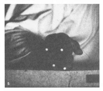
block are in contact for five milliseconds. As the fist strikes the block it decelerates rapidly. The change in the positions of the dots with respect to one another indicates that the fist is compressed and distorted to such an extent that it scarcely acts like a solid object. Hence models of the impact process cannot consider the fist as being solid.
