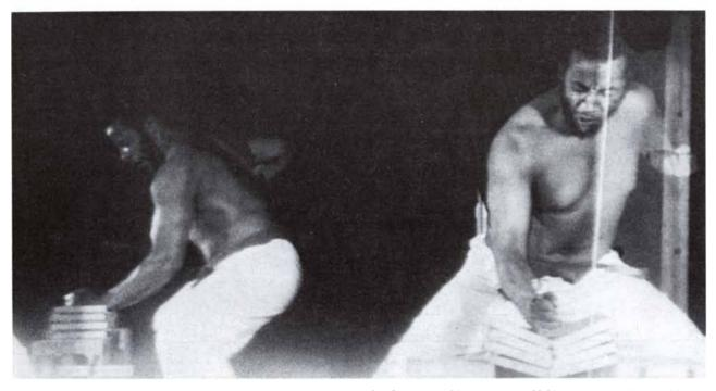
ROTATING-DRUM CAMERA provided simultaneous side and front views of a hammer-fist strike, in which the fist is brought down from above the head in a circular arc. Here the fist is breaking four
