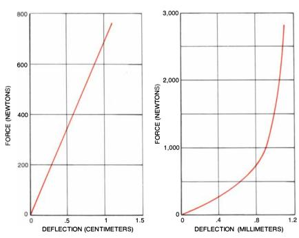
HYDRAULIC-PRESS MEASUREMENTS were made of the deflection of a wood block (*left*) and a concrete block (*right*) as a function of the applied force. Each of these plots yielded values for the elastic modulus, which for a given material is a constant that indicates its springiness, and for the modulus of rupture, which is the minimum stress that causes a block to snap. It is useful to know these moduli in order to find the energy needed to break each kind of block.
