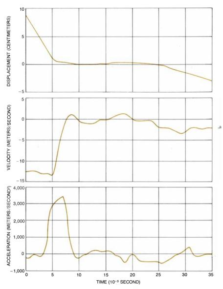
VERTICAL DISPLACEMENT, velocity and acceleration are plotted for the dot at the lower right on the fist in the photographs on the opposite page. The peak deceleration of the dot was 3,500 meters per second squared; that of the other dots was 4,000 meters per second squared.
